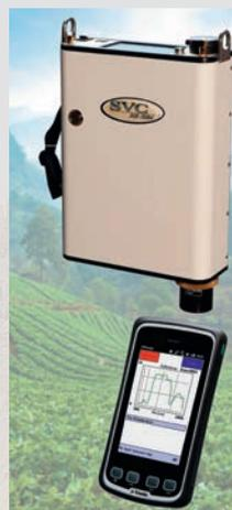
▲ Example of a recent portable spectroradiometer (SVC HR-768si) for measuring reflectance in the visible to medium infrared range.
