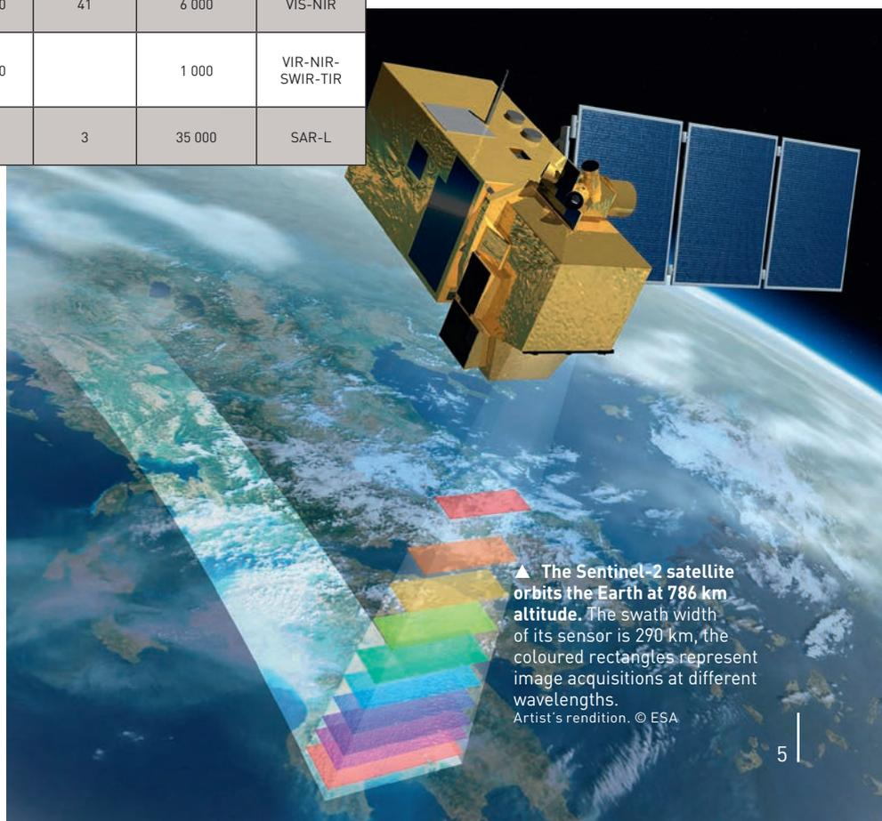
▲ The Sentinel-2 satellite orbits the Earth at 786 km altitude. The swath width of its sensor is 290 km, the coloured rectangles represent image acquisitions at different wavelengths. Artist's rendition. © ESA
